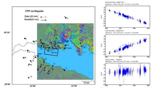
Fig. 6. The region of the earthquake on 15.06.1995 with determined by GNSS and InSAR methods of coseismic deformations. The assessed and modelled displacements are presented respectively by thin and thick arrows. On the right is presented a comparison between permanent stations on the two coasts of Corinth Bay. The space vectors between stations on the two coasts of the bay has been struck.
