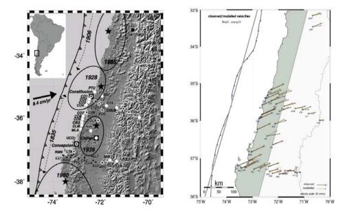
Fig. 9. On the left – Geodynamic GNSS network of 41 points in the seismogenic zone of Central Chile with the results of monitoring from 1996, 1999, and 2002. On the right (in grey) – the zone of collision of the Pacific Nazca Plate with this in South America, obtained from the modeling of interseismic displacements.
