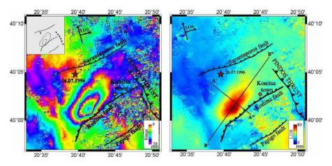
Fig. 7. Seismogenic zone of town of Konitsa and the faults activated with the assessed coseismic deformations with InSAR of the earthquake of 1996
